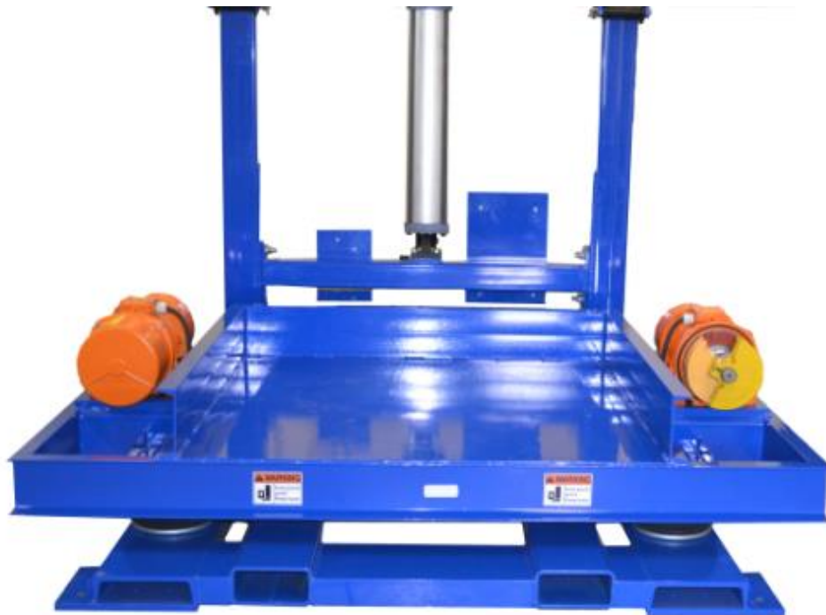
Figure 5 - Vibratory Flat Deck (Standard) pictured with Hydraulic Lift Cylinder option
