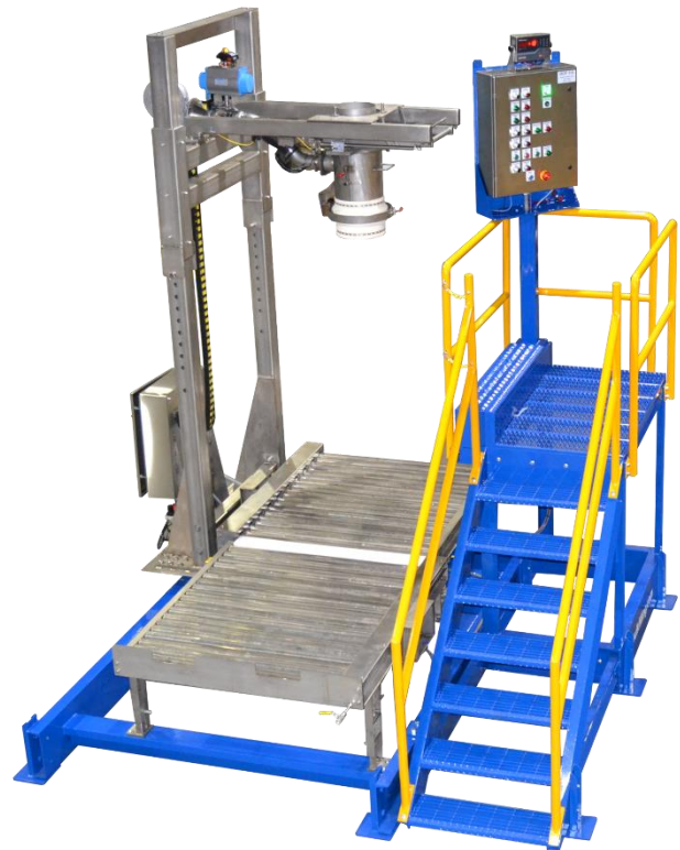
Figure 19 - Custom Stainless Steel DensiMAX™ with Nema 4X Enclosure, 100% simple relay-based controls and digital weight indicator. Specifically designed for outdoor use in extreme weather conditions.
