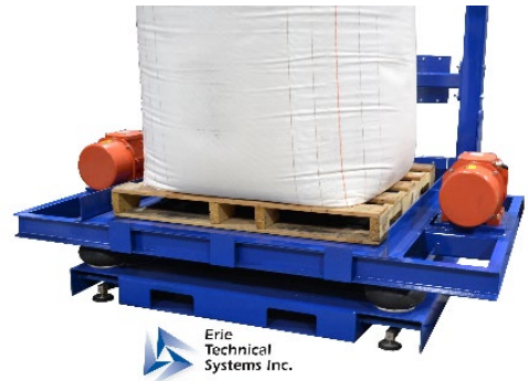
Figure 15 – Vibratory Flat Deck with Bulk Bag
